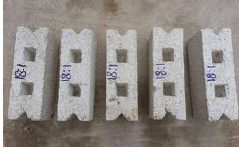
Figure 1. Five bricks samples as 18:1 ratio Figure 2. Five bricks samples as 6:1 ratio
