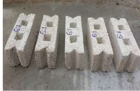
Figure 1. Five bricks samples as 18:1 ratio Figure 2. Five bricks samples as 6:1 ratio
