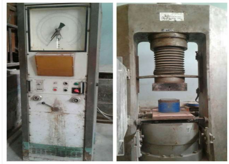
Figure 5. Compressive testing machine (250)
